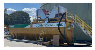
NPE's conditioning tanks have been designed, built and certified at NPE to assist with our solids processing solutions. The design allows top loading of the tank for various configurations including 2 x 20ft skids or a single 40ft processing skid. With its unique design, allows NPE the flexibility to provide a full turnkey screening and separation solution for our customers based on the site and material requirements whilst ensuring a reduced footprint.
