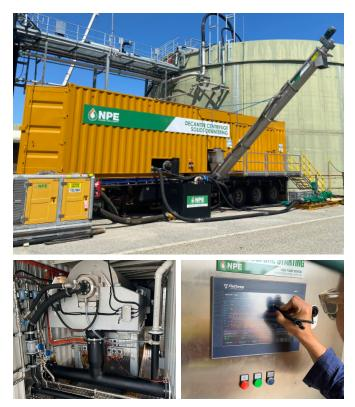
This system ensures the removal of rag and grits from the biosolids before they are removed from site. This allows more options for disposal of the biosolids via beneficial reuse solutions without the concern of contamination within the final product and avoids the need to take the material to landfill. We have maintained a minimum 20% solids content for all material processed through our new mobile centrifuge which has ensured safe and efficient transport solutions when disposing from site.
