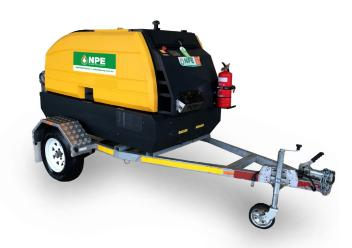
The SPP AUTOPRIME QC200-200mm pump is a fully enclosed diesel driven pump unit with high efficiency, designed to pump most liquids including sewage and semi solids. The enclosure provides sound reduction and security for use in noise sensitive areas.
