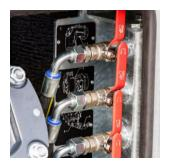
Central flushing system The BV series comes standard with a central flushing system to keep your sludge pump in optimal condition.
