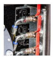
Central flushing system The BV series comes standard with a central flushing system to keep your sludge pump in optimal condition.
