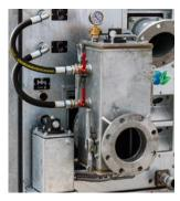
"Easy clean" floating boxes Two fully galvanised floatingboxes with stainless steel floaters are easy to clean after the job is done.
