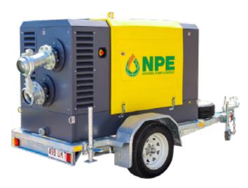
The pump system consists of a centrifugal pump and a vacuum pump - making automatic priming possible. Even with suction heights of several meters the machine rapidly evacuates the air from the suction pipe and starts to pump. Additionally, thanks to the semi-open impeller, the PAS MF range is also suitable for pumping liquids with solids in suspension.
