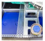
**Fully bunded unit** Fully bunded unit eliminating fuel/oil and AdBlue® spills at all times.
