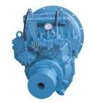
Ratio transmission gearbox Hydraulically actuated clutches and helical gearing for a smooth operating speed reduction between engine and pump.
