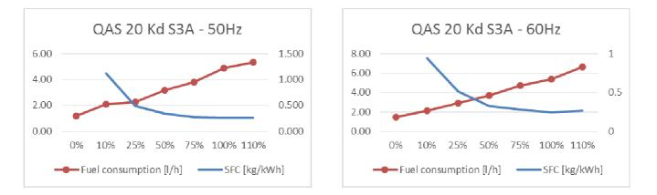
(Reference conditions at 25% Air Inlet Temperature, 60% Relative Humidity, 1bar Absolute inlet pressure, for different conditions or limitations contact Atlas Copco technical support).
